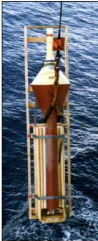
Figure 4.1.3.1.1 Deployment of a FGGE type buoy
